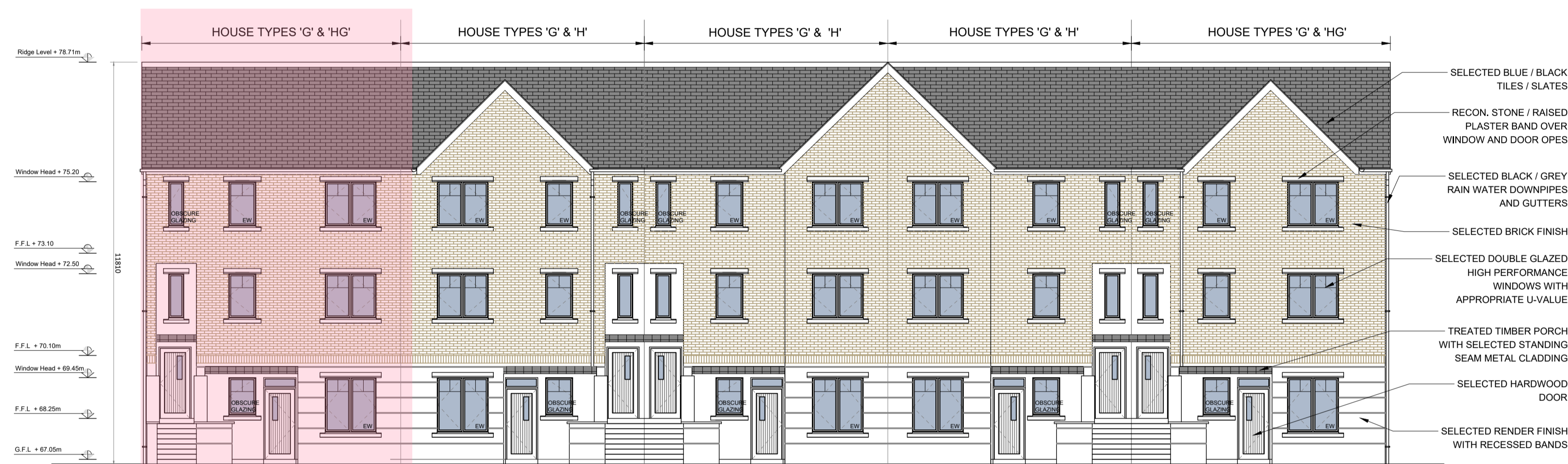
EAST ELEVATION - BLOCK G
